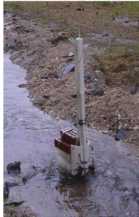
Figure 3-2. Siphon sampler
