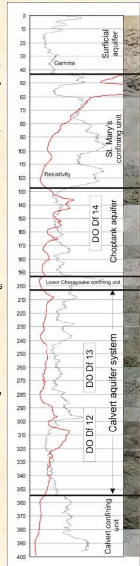
The completed wells were airlifted to remove drilling fluid and to develop the well screens. DO Df 13 could not produce enough water to be properly developed and tested. Twenty-four hour aquifer tests were conducted on DO Df 12 and 14 at constant rates of 101 gallons per minute (gpm) and 8.6 gpm, respectively. During each test, there was little or no observable change in water levels in the observation wells as a result of pumping from the test well.
