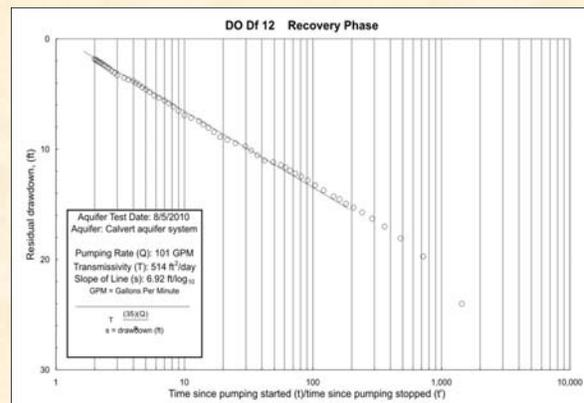
Transmissivities calculated by the Cooper-Jacob method for the recovery phase of the tests were 514 ft<sup>2</sup>/day for DO Df 12 and 28 ft<sup>2</sup>/day for DO Df 14.
