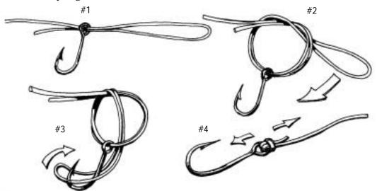
**NON-SLIP LOOP KNOT** – This knot creates a fixed loop so that a hook can freely move. It is best with larger lines where a tight knot such as the Improved Clinch can impede the hook/bait or lure movement. It is similar to tying the Improved Clinch Knot.
