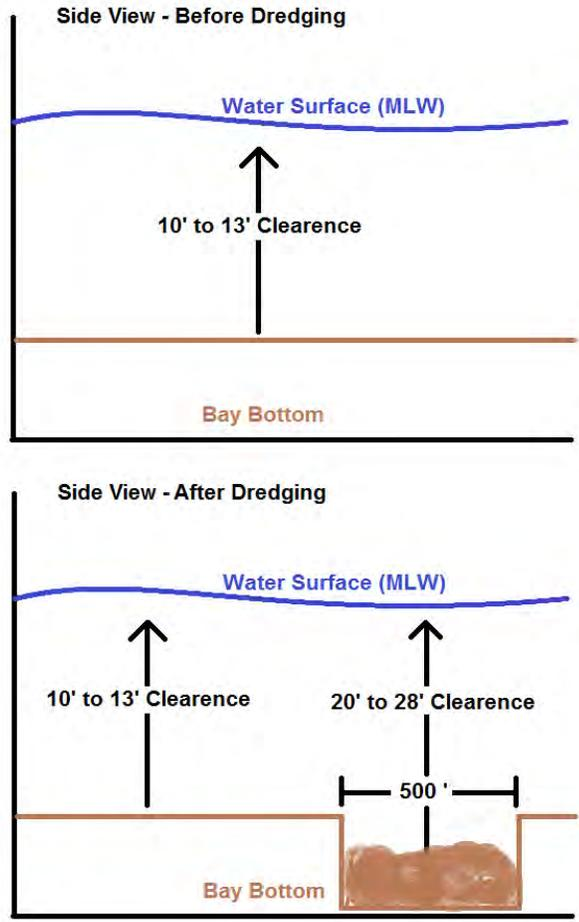
Figure 1b. A typical cross section of the proposed dredge cuts made at Man-O-War shoal.
