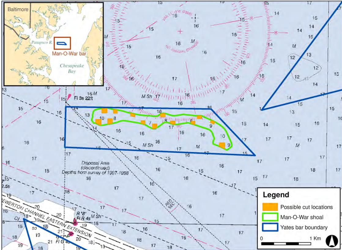
Figure 1a. The location and general shape of Man-O-War shoal. Dark lines indicate the boundaries of oyster bars mapped by Yates (1911). Yellow rectangles within the outline of the shoal illustrate the types of cuts anticipated as shell is removed by dredging along the perimeter.
