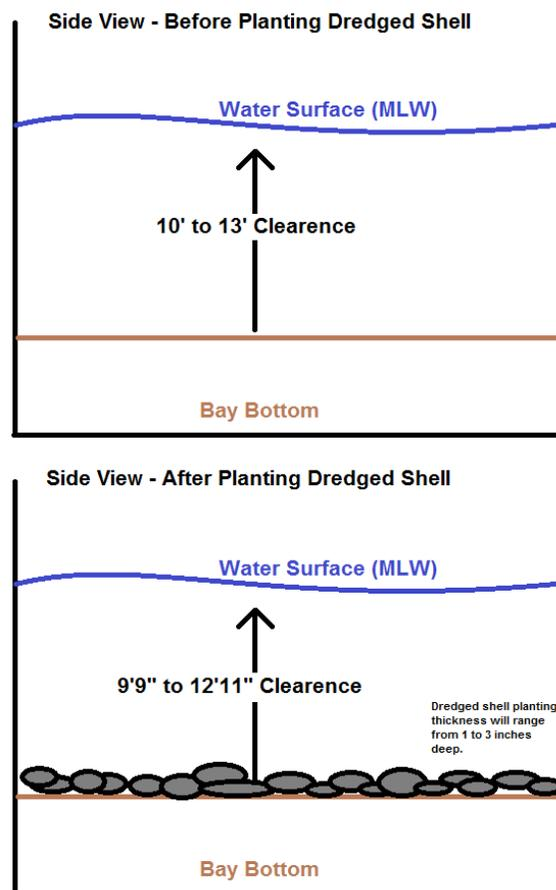
Figure 14: A typical cross section of planting dredged shell.
