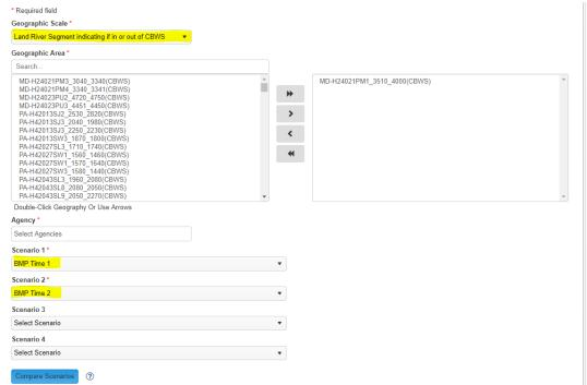
10) In the result of this, click on the loads tab to compare the difference in loads between the two scenarios. Use the difference in Edge of Stream values (highlighted values below) as the load reduction achieved via adding treatment volume to your wet pond. For example, there is a difference of 222 lbs of Nitrogen between scenario 1 and 2 in the below example.
