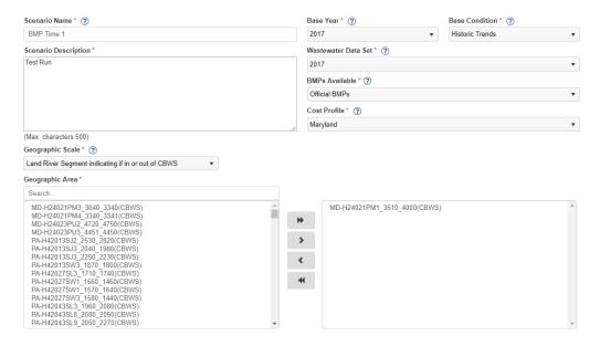
4) Press edit under the scenario you just created and navigate to the developed BMPs tab. Under developed BMPs, pick Stormwater performance Standard- Stormwater Treatment, filling out the parameters and acre feet storage of EXISTING water quality treatment. Click save when finished.
