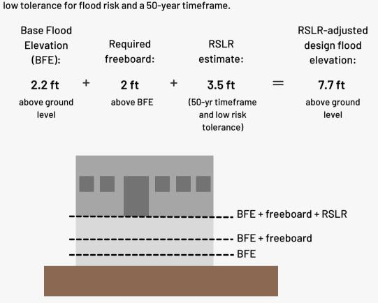
Example: Determining the design flood elevation for a structure in Cambridge, MD with
