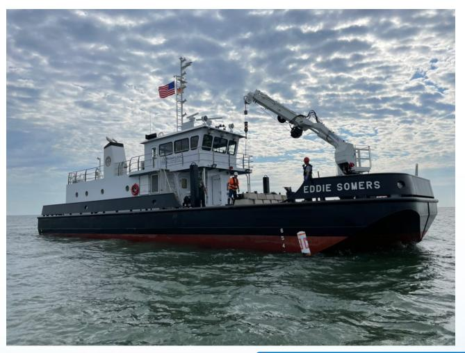
M/V EDDIE SOMERS / Service Area BUILT: Blount Boats (2022) LENGTH: 94' WIDTH: 27" DRAFT: 5" 188 TON ICE BREAKING CAPABILITIES: 18" PROPULSION: 1,500 HP TWIN SCRW DIESEL ENGINE
